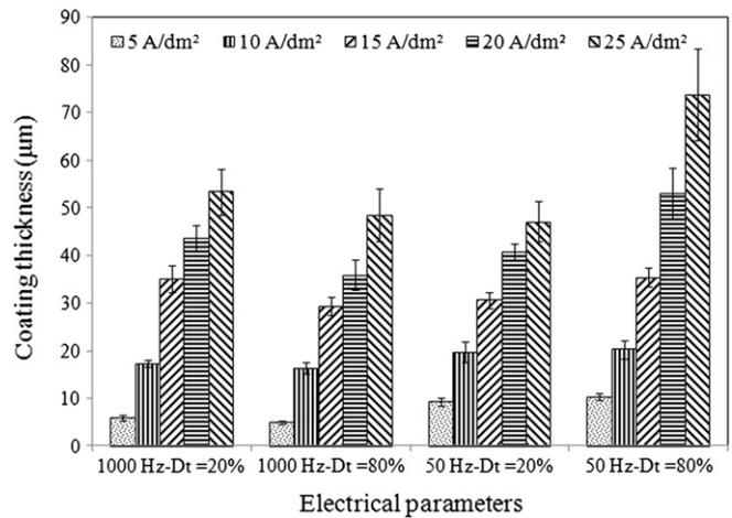
Fig. 3. Effect of electrical parameters on coating thickness of PEO treated 6061 aluminum alloy substrates.
