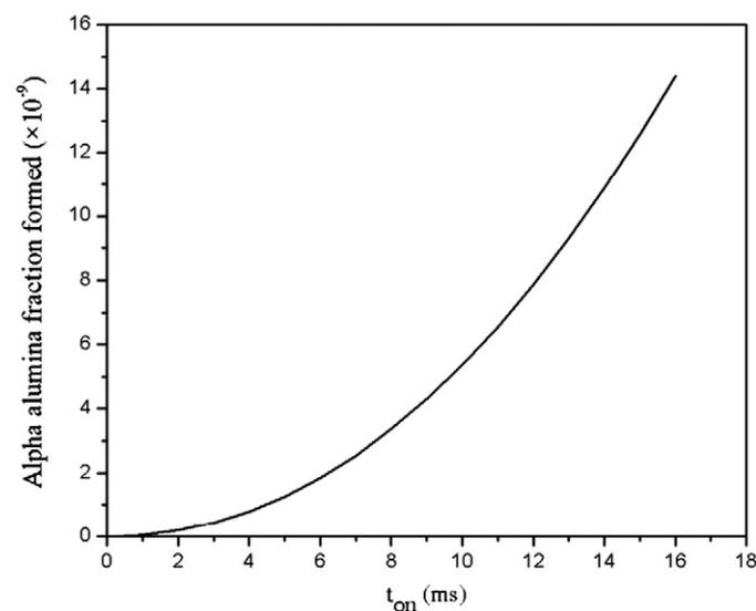
Fig. 8. Variation trend in the fraction of formed  $\alpha$ -alumina in a single pulse as a function of  $t_{on}$  calculated using KJMA equation assuming an isothermal transformation temperature of 1050 °C.
