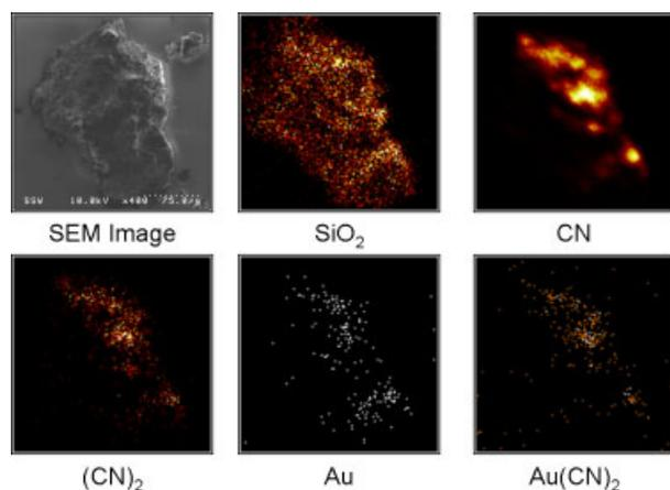
**Figure 1.** SEM image and TOF-SIMS elemental and compositional maps for carbonaceous particle from CIL tails sample. The quantified amount of metallic gold on this particle was 4.5 ppm while the amount of Au as Au(CN)<sub>2</sub> compound gold was 38.1 ppm.
