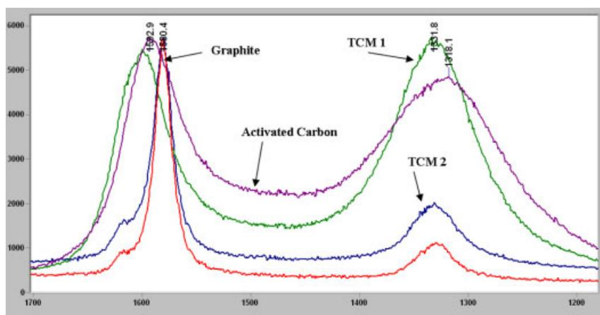
**Figure 2.** Comparative Raman spectra from two reference materials (graphitic carbon and activated carbon) and two TCM particles from CIL tail sample.
