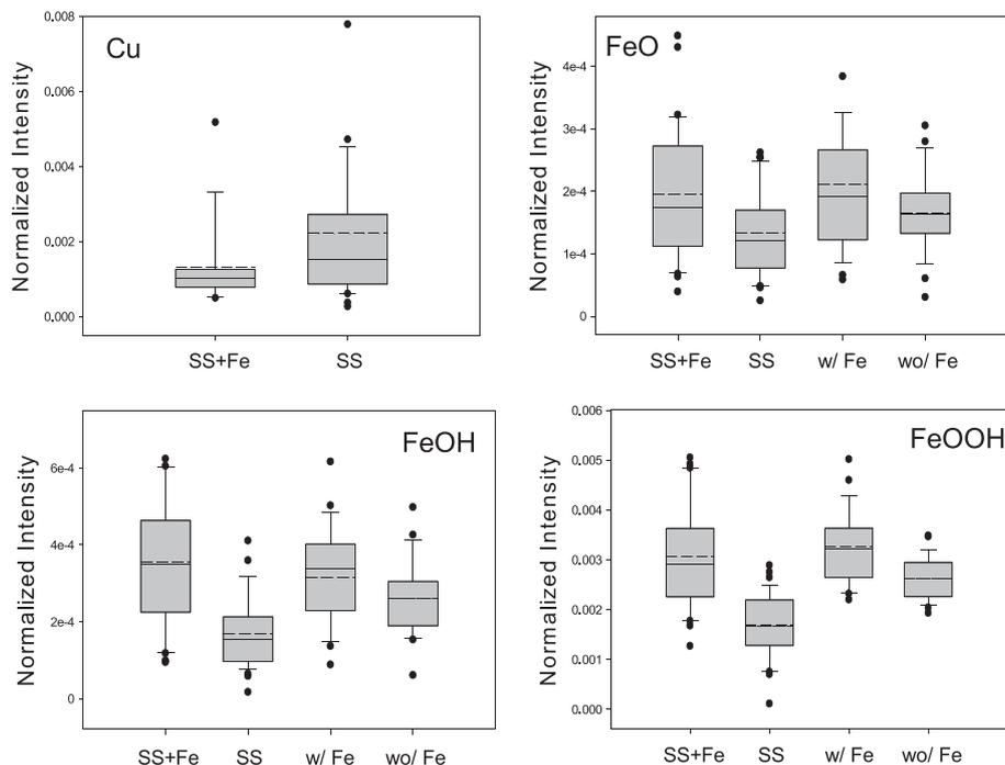
**FIGURE 6** Normalized intensity of surface copper and iron oxyhydroxyl species on sphalerite surfaces during grinding with (shown in the picture as SS + Fe) and without (SS) the addition of FeSO<sub>4</sub>. Also shown are normalized intensity of iron oxyhydroxyl species on sphalerite surfaces from bench scale testing at the plant; tests with FeSO<sub>4</sub> (W/Fe) and without FeSO<sub>4</sub> (WO/Fe). All tests were performed at addition rates of 600 g/t of FeSO<sub>4</sub>
