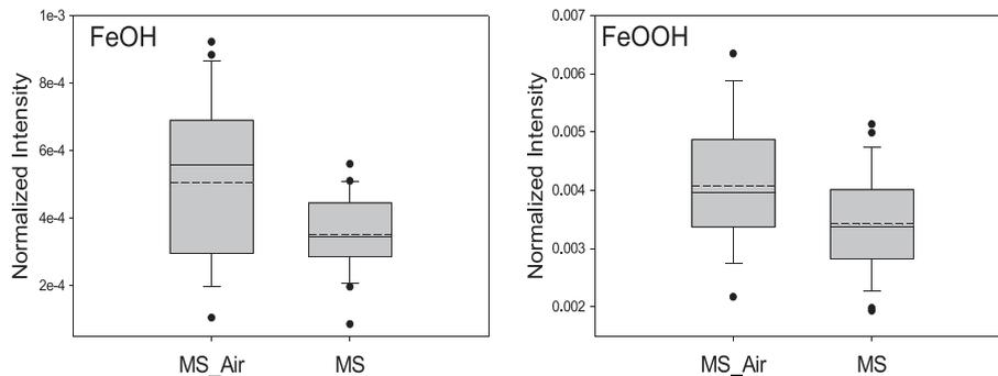
**FIGURE 5** Normalized intensity of iron oxyhydroxyl species on sphalerite surfaces in grinding with air sparged ball mill (MS + Air) and without air sparging (MS)
