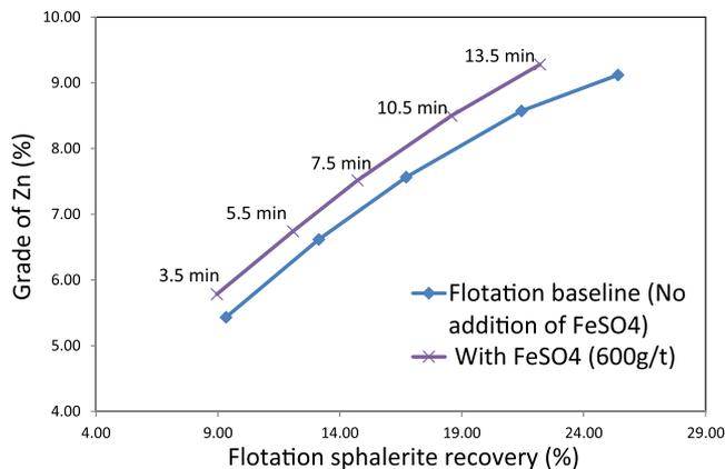
**FIGURE 7** Bench scale flotation of sulphide ore with and without 600 g/t FeSO<sub>4</sub>
