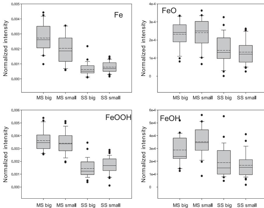
**FIGURE 3** Normalized intensity of Fe and iron oxide and oxyhydroxide species on sphalerite surfaces as measured by TOF-SIMS. Abbreviations are given in Table 1
