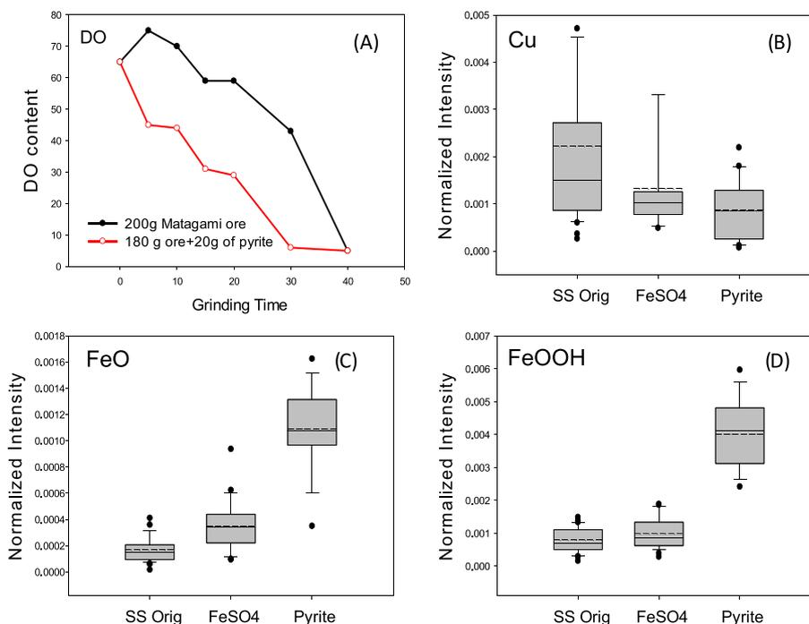
**FIGURE 8** (A) Measured DO content in grinding tests with the Matagami ore and 20% pyrite increase in the same ore. (B), (C), and (D) Surface Cu, FeO, and FeOOH species on sphalerite surfaces as measured by TOF-SIMS. Abbreviations are as follow: no additions milling with stainless steel only (SS orig), milling with addition of FeSO<sub>4</sub> (FeSO<sub>4</sub>), and with addition of 20% pyrite (pyrite)
