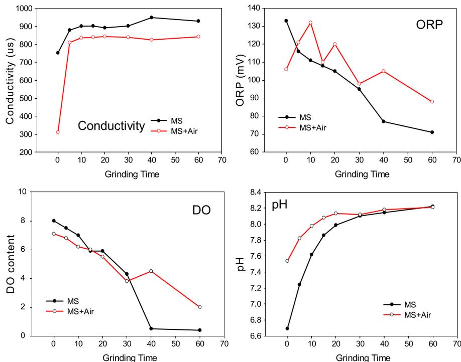
**FIGURE 4** Pulp chemistry variations during grinding with air sparged ball mill (MS + Air) and without air sparging (MS)
