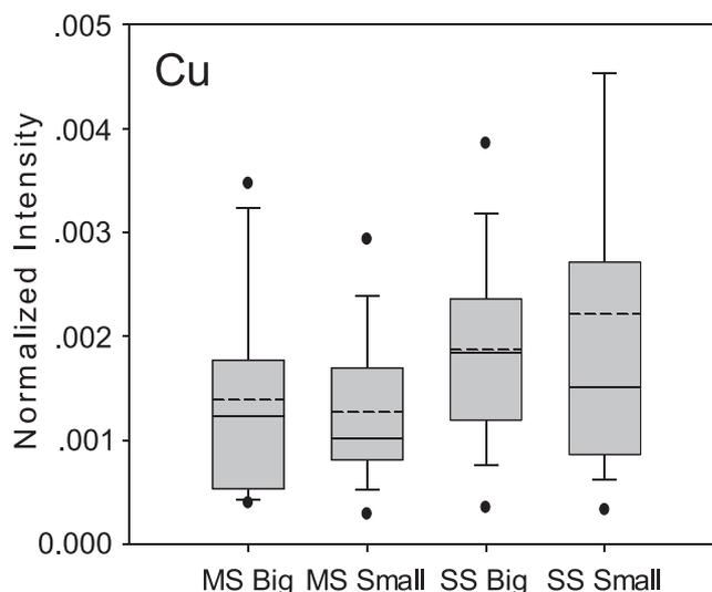
**FIGURE 2** Normalized intensity of Cu on the surface of sphalerite as measured by ToF-SIMS. Abbreviations are given in Table 1
