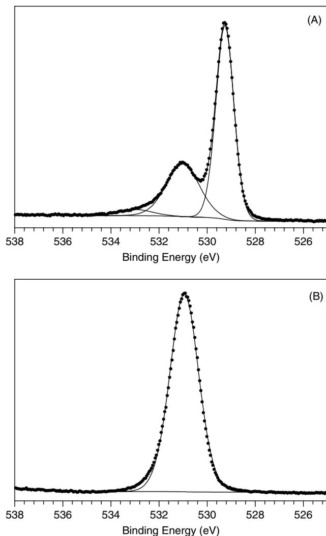
**Figure 1.** O 1s spectra of (A) NiO and (B) Ni(OH)<sub>2</sub>.
