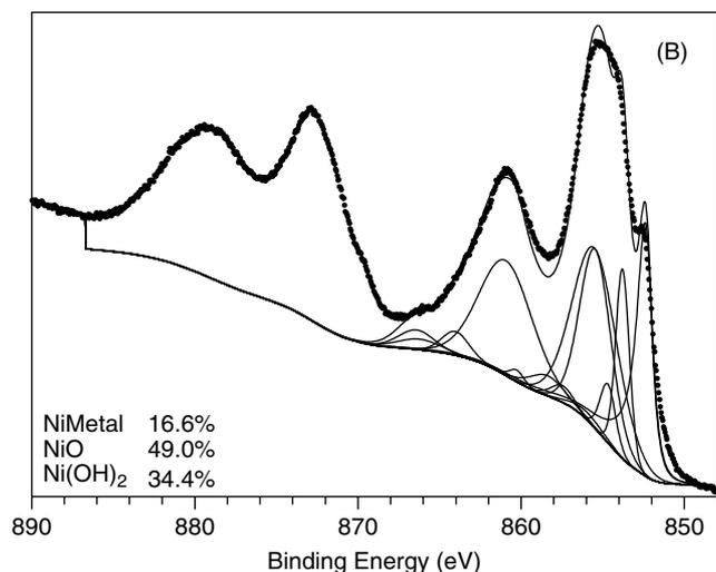
**Figure 4.** Ni 2p spectra of INCO (Type 123) nickel powder (A) and an ultrafine nickel powder (B) A Shirley background under the entire Ni 2p spectrum with an offset on the higher binding energy endpoint is used for both spectra.
