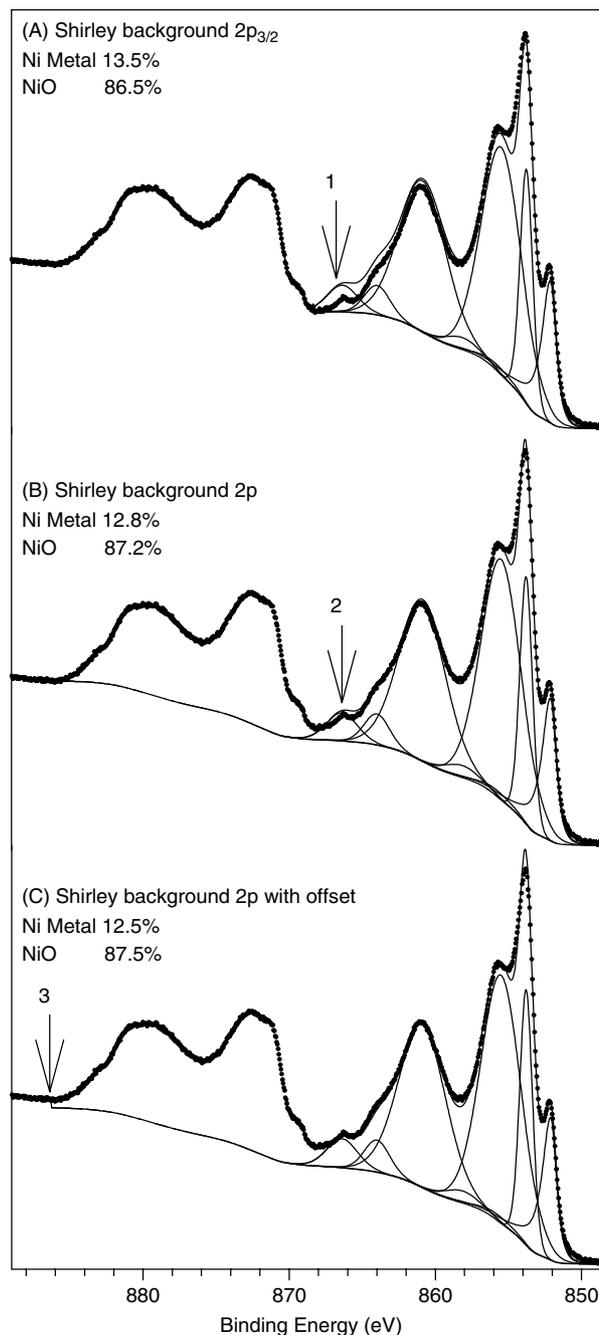
**Figure 2.** Ni 2p thin oxide film spectra. (A) Shirley background under only the Ni  $2p_{3/2}$  portion of the spectrum. (B) Shirley background under the entire Ni 2p spectrum. (C) Shirley background under the entire Ni 2p spectrum with an offset on the higher binding energy endpoint.
