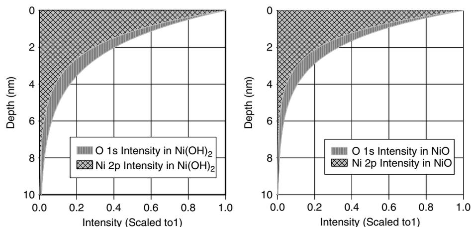
**Figure 7.** Models of the O 1s and Ni 2p photoelectron intensity as a function of depth for Ni(OH)<sub>2</sub> (left) and NiO (right).
