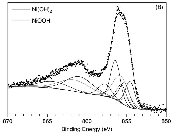
**Figure 5.** Ni 2p<sub>3/2</sub> portions of the Ni 2p spectra of  $\gamma$ -NiOOH (A) and  $\beta$ -NiOOH (B). The Ni(III) spectral shape for  $\beta$ -NiOOH is modeled after that of the  $\gamma$ -NiOOH spectrum and the Ni(II) components are modeled after that of Ni(OH)<sub>2</sub>.
