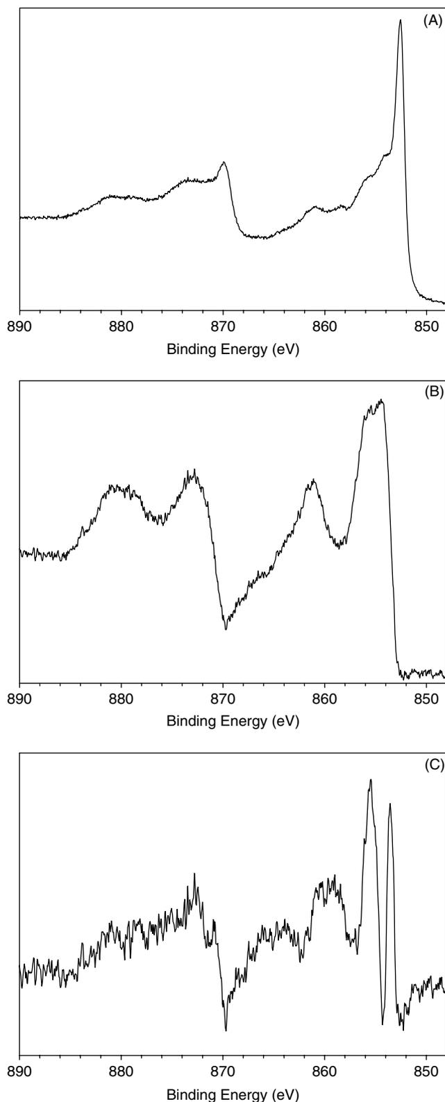
**Figure 6.** Ni 2p spectra from (A) Ni metal surface covered by a thin NiO film; (B) after subtraction of the metal spectral components and (C) after subtraction of the metal and NiO spectral components.
