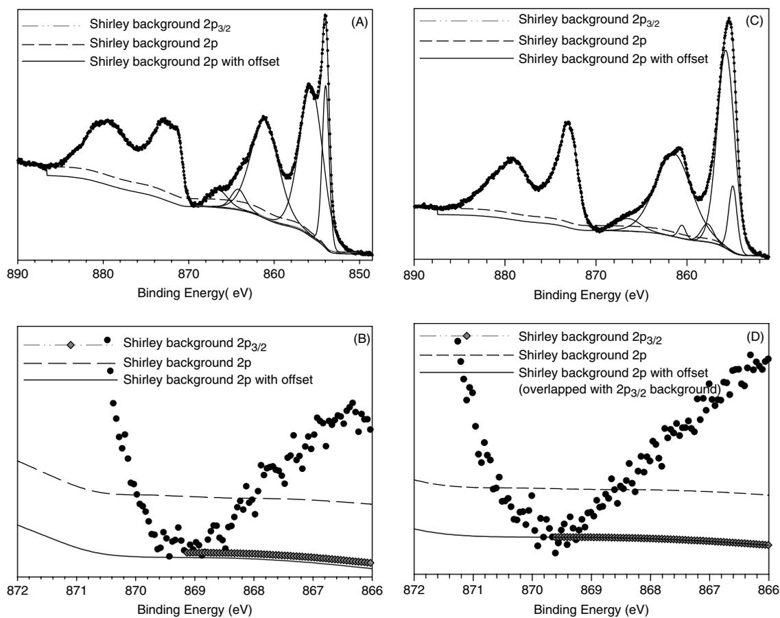
**Figure 3.** Ni 2p spectra of NiO (A) and (B) and Ni(OH)<sub>2</sub> (C) and (D) showing three different Shirley background configurations. Figures (B) and (D) provide detail on the backgrounds at the low intensity region between the Ni 2p<sub>3/2</sub> and Ni 2p<sub>1/2</sub> portions of the spectra for NiO and Ni(OH)<sub>2</sub>, respectively. The fitted peaks use the Shirley background across the 2p<sub>3/2</sub> portion of the spectra.
