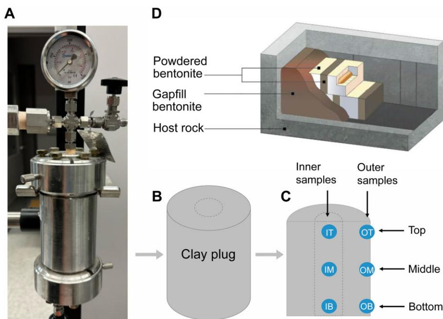
**Figure 1.** Photograph of a pressure vessel (A) and schematic of the clay plug within the pressure vessel (B) and the sample layers sampled: top, middle, and bottom of the inner core and the outer layer (C). Pressure vessels are filled with powdered or gapfill bentonite clay, the former being the raw material processed to produce HCB and GFM, which are both components of the theoretical design of a DGR (D; modified from King et al. 2017).
