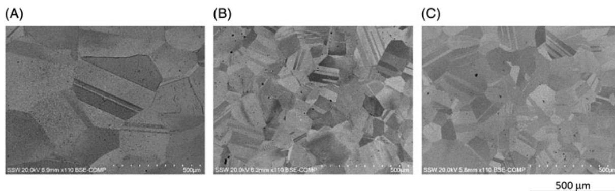
**Figure 2.** SEM images of the three alloys after critical crevice solution immersion (a) G-30, (b) C-22 and (c) BC-1.
