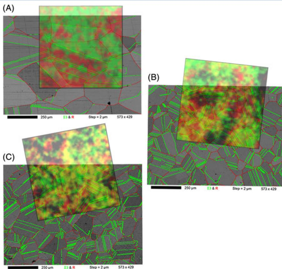
**Figure 5.** Overlaid XPS survey images of molybdenum (red), chromium (green) and mixed (yellow) with the electron backscatter diffraction images for (a) G-30, (b) C-22, (c) BC-1 showing  $\Sigma 3$  and random grain boundaries.
