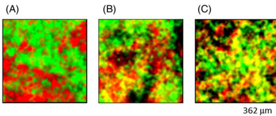
**Figure 4.** Overlaid XPS survey images of molybdenum (red), chromium (green) and mixture (yellow) for alloys (a) G-30, (b) C-22 and (c) BC-1.
