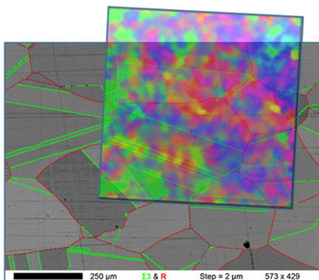
**Figure 7.** Overlaid XPS images of Mo metal (red), Mo IV (blue) and Mo VI (green) for sample G-30 superimposed with the electron backscatter diffraction image showing the  $\Sigma 3$  and random grain boundaries.
