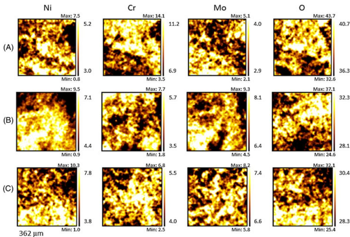
**Figure 3.** Elemental XPS survey images showing Ni, Cr, Mo and O for each alloy after critical crevice solution (a) G-30, (b) C-22 and (c) BC-1.
