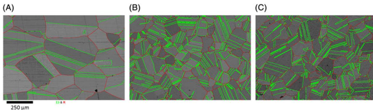
**Figure 1.** Electron backscatter diffraction band contrast images for alloys before corrosion in critical crevice solution (a) G-30, (b) C-22 and (c) BC-1. The  $\Sigma 3$  boundaries are green, while the random boundaries are red.
