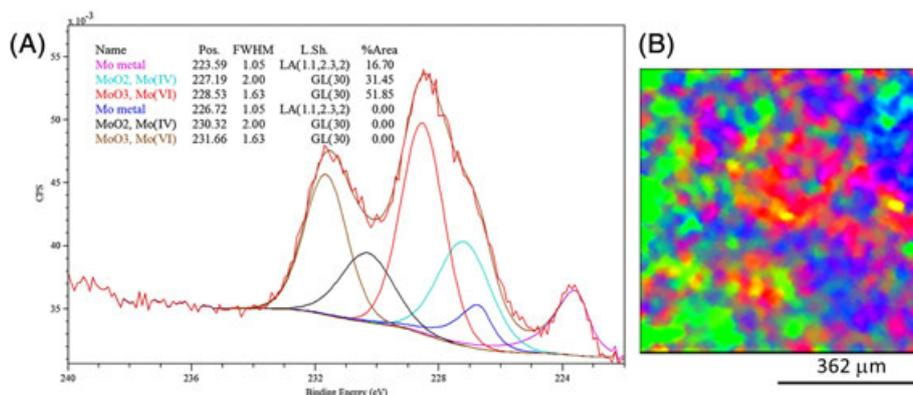
**Figure 6.** (a) High resolution Mo 3D spectrum and (b) overlaid XPS images for Mo metal (red), Mo(IV) (blue) and Mo(VI) (green) for G-30.
