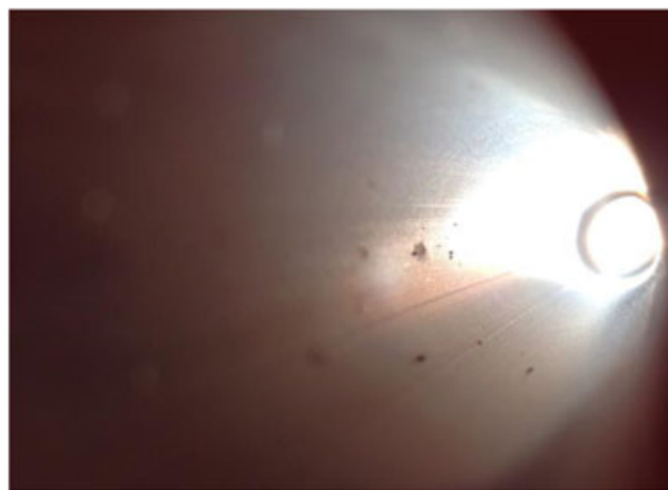
Figure 8. Back-lit macrograph of a tube interior from L1. Many micro protrusions of differing size are visible. [Colour figure can be viewed at wileyonlinelibrary.com ]
