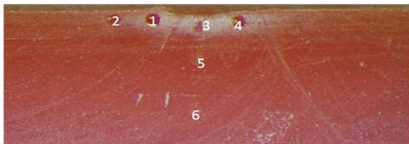
Figure 5. Optical micrograph of the crack face of failure L1–2. The tube inside diameter is at the top of the image, and the image covers the outermost 10% of the tube diameter. About 80% of tube diameter was cracked by the action of chemical attack and the remainder by mechanical forces. The numbers indicate positions where microscopic Fourier transform infrared spectra were obtained. Carbonyl indices for positions (1–6) are 0.19, 0.19, 0.19, 0.20, 0.24, and 0.24. The crystallinity ratio for positions (1–6) are 0.50, 0.56, 0.52, 0.52, 0.66, and 0.65. [Colour figure can be viewed at wileyonlinelibrary.com ]
